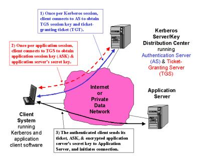
The Kerberos Server/KDC has two main functions known as the Authentication Server (AS) and Ticket-Granting Server (TGS). The steps in establishing an authenticated session between an application client and the application server are:
